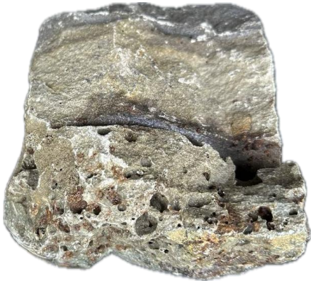
Fig. 1. Hadfield Steel slag particle from Navoi Machine Building Plant.
