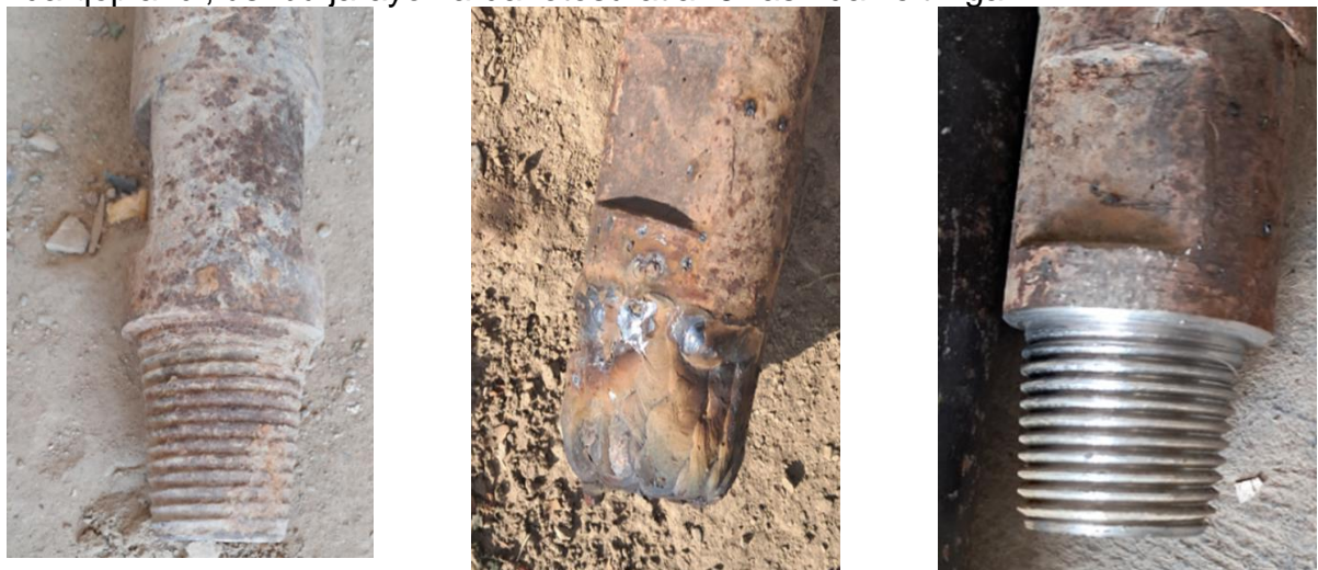
a - qayta tiklanadigan namuna, b - elektr yoyli payvandlab eritib qoplangandan so'nggi holat, v - rezba ochilgandan so'nggi holat.
